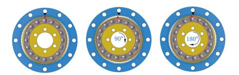
Example: with 100:1 ratio, 100 clockwise input motor rotations results in 1 counterclockwise output rotation.
